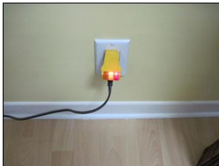
Reversed polarity on bedroom outlet 5089
